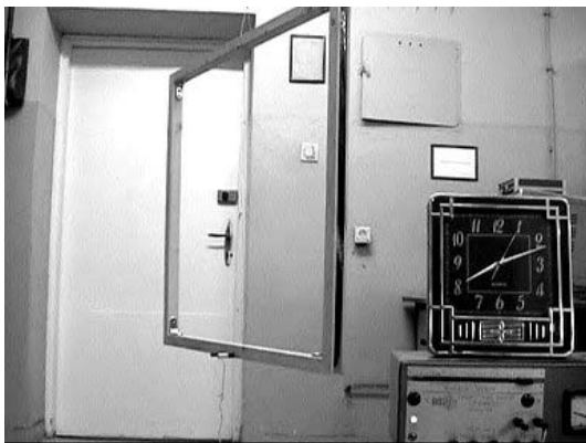
Photo 3. Helmholtz coil (a winding of about 100 turns of 1 mm diameter copper wire) can be used for: a) showing the force momentum acting on it if the electrical current (3-5A) is supplied; b) the Faraday-Lenz current (a few meV), when turned around.
