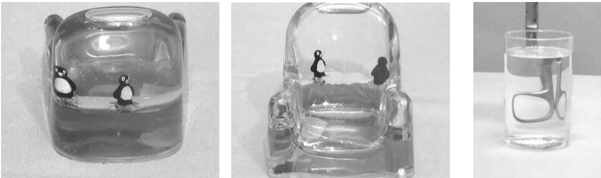
Photo 7. Diopters (semi-lenses) – photo a) and b) and a cylindrical thick lens (a glass of water). a) and b) – this is a chair-like support for mobile telephones – with two penguins floating inside; the backside of the chair is convex on one side and concave on another, with the curve radius changing: the size (horizontal) of penguins depend on their position and the directions of observation. c) a cylindrical lens changes the size only in one dimension; in a thick lens the magnification depends much on the position of the object relative to the optical axis. This what is called an “aberration” (spherical) for thin lenses becomes dominant for thick lenses.
